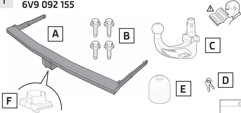
The cover cap for the mounting recess (F) is located in the recess in the tow bar mounting recess.
