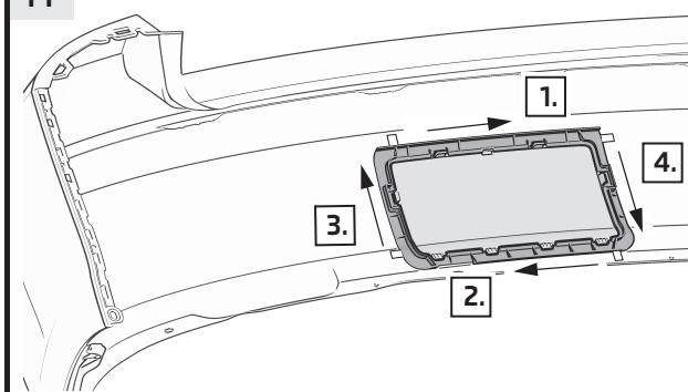
Remove the protective sheet from the double-sided adhesive tape in the sequence shown in the figure. This must be carried out with extreme care.
