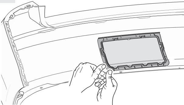
Carefully press on the bonded frame along the entire length of the adhesive surface.
